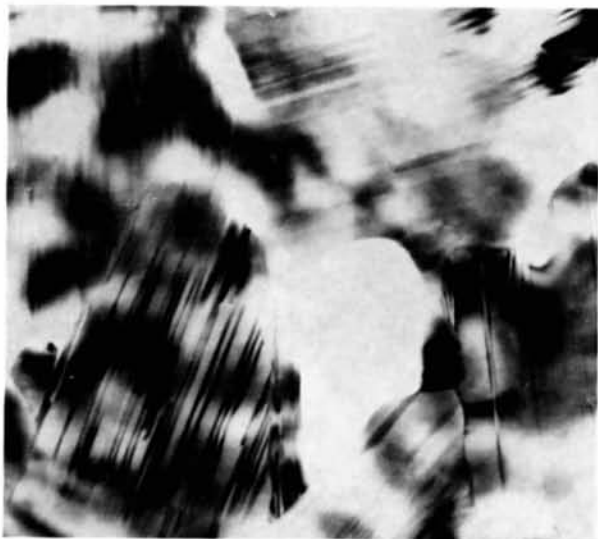
Fig. 5. Faulted region which gave the sixfold modulated pattern of Fig. 7 (Magnification 40,000).
