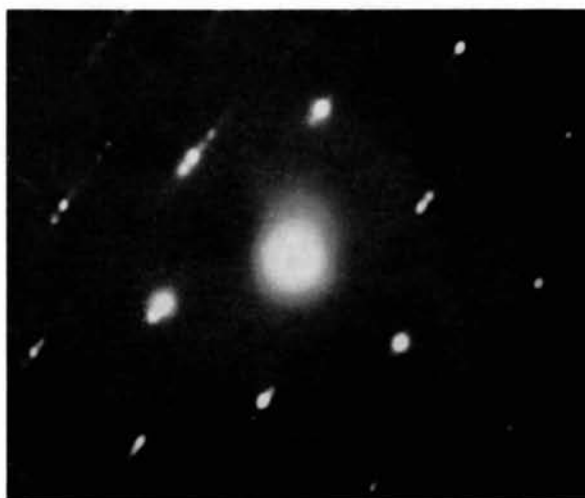
Fig. 8. Single-crystal pattern showing additional spots when the featureless region shown in Fig. 4 was slightly tilted.
